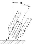
◆ bend the welding element (1) with the bending device once by 30° in any direction.
