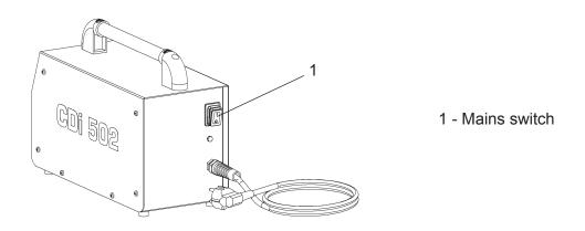
The switch for mains mode is located on the rear of the stud welding machine.
