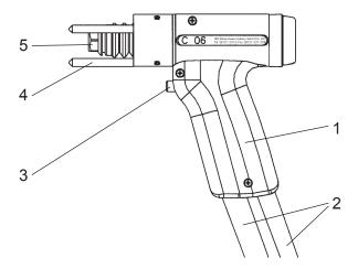
The body of the welding gun consists of a sturdy two-part plastic housing.
