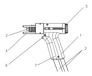
The body of the stud welding gun consists of a sturdy two-part **plastic housing (1)**.
